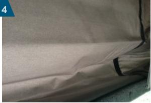
Continue to lower the roof whilst slowly pulling down the straps in increments of about 4 inches (100mm)
