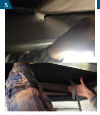
Continue to lower the roof whilst slowly pulling down the straps in increments of about 4 inches (100mm) until the roof is fully closed.
