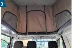
Fully close the scenic opening using the zip fasteners which run horizontally around the roof.
