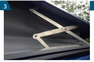
Hold both loose straps and slowly pull the roof down in increments of about 4 inches (100mm).
