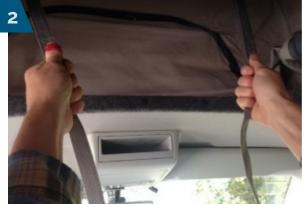
Re-attached the elastic strap, this can be done by standing on the front seats and leaning into the bed space.
