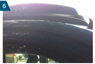
When the roof is fully lowered, step out of the vehicle and check that the canvas is not visible at any point from the outside.
